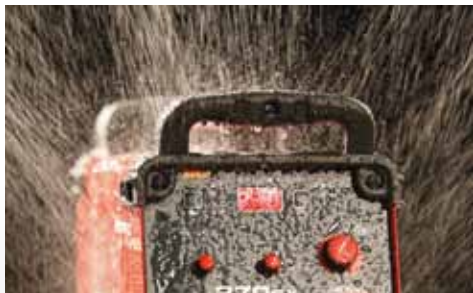
IP testing in the Lincoln lab
